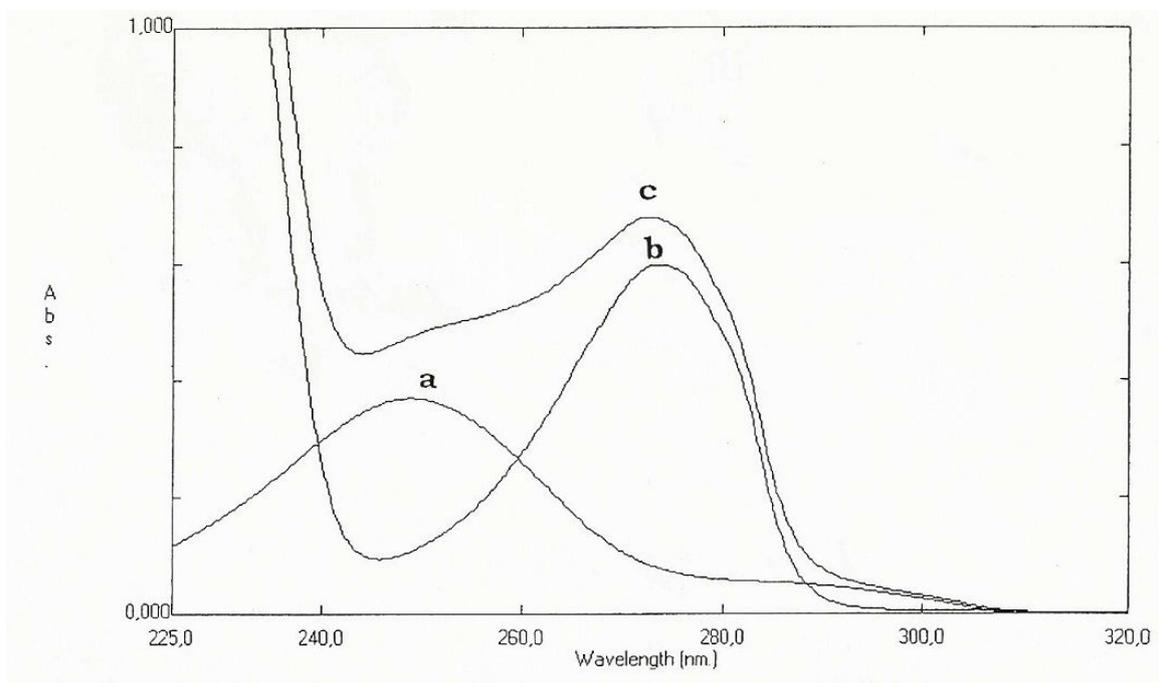
**Figure 1.** Zero-order absorption spectra of a) 3  $\mu\text{g/mL}$  solution of paracetamol, b) 20  $\mu\text{g/mL}$  solution of methocarbamol in methanol c) solution of 3  $\mu\text{g/mL}$  paracetamol + 20  $\mu\text{g/mL}$  methocarbamol mixture in methanol
